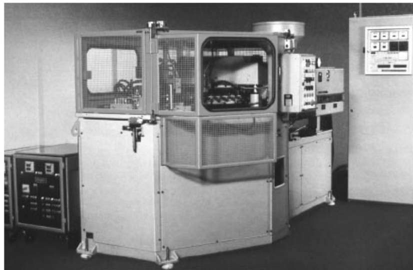
Fig. 2. Three-station injection blow-molding machine utilizing a horizontal reciprocating screw produced by Bekum, Berlin, Germany.
