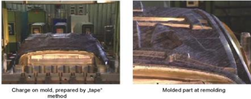
Fig. 4 Molding and remolding of experimental decklid
