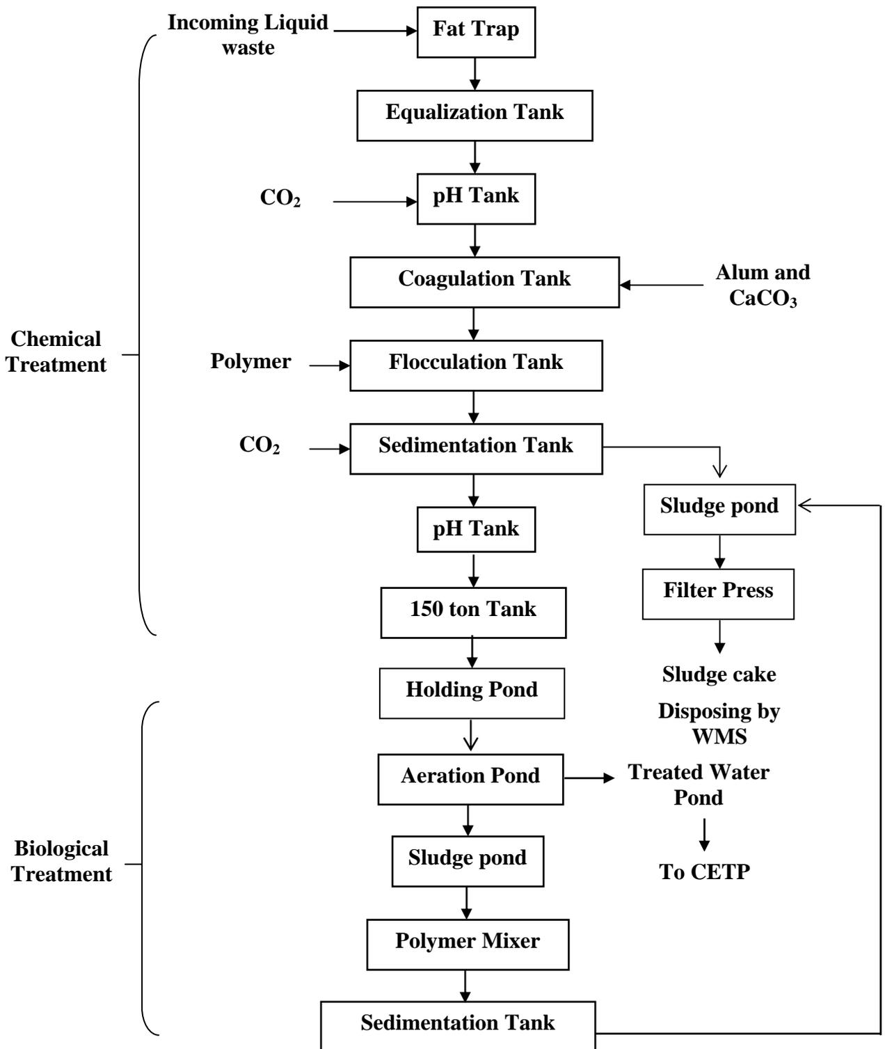
Figure 6- Wastewater flow diagram
