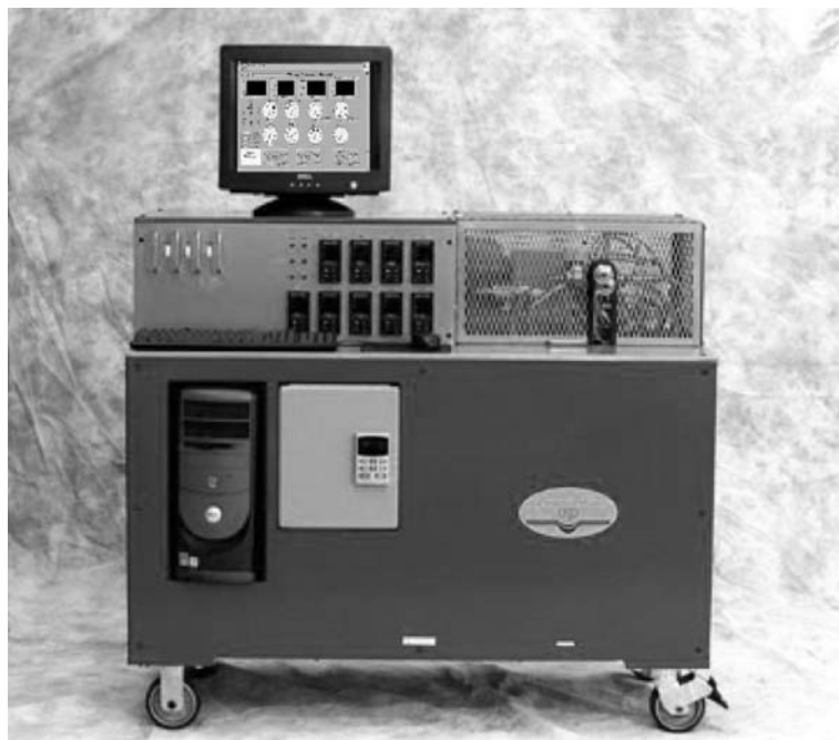
FIG. 4.13 CEP Lodge Stressmeter. (Courtesy of Chemical ElectroPhysics Corp.)
