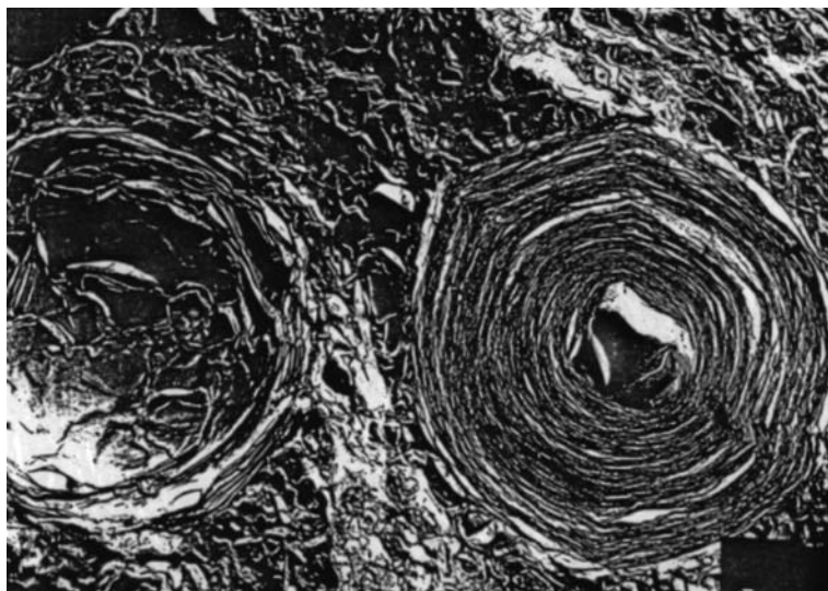
FIG. 12.8 Electron micrograph of a DHTDMAC aqueous dispersion. An intact vesicle is seen on the left, a cross section on the right, in which the lamellar structure is apparent (freeze fracture, magnification \times 2500 ).
